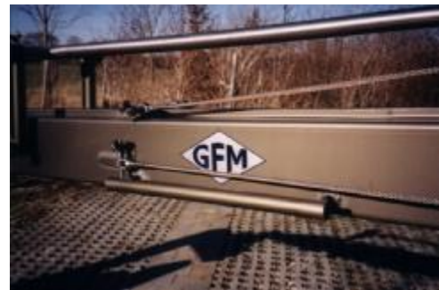
Rigging rod connected to crane arm
